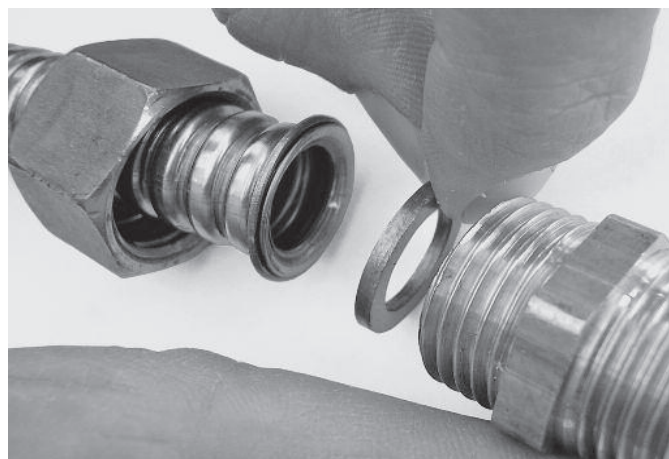
Fig. 6 Insertion of Cu-seal between flanged rim and body of fitting
