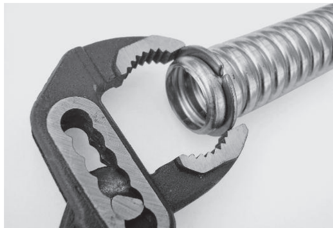
Fig. 4 Attaching the clamping ring
